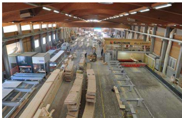
Manufacture : unique CNC machine with 3 robots for beams until 40m length and 5m wide, lathe for \varnothing 1,20m pieces
